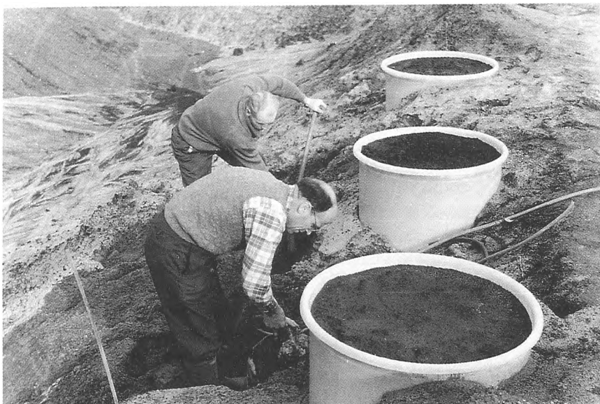
Fig. 2. Lysimeters used by Kjeld Rasmussen in studies of pyrite oxidation.
